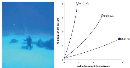
Fig. 8. “underwater weather balloon” reaction to varying current speeds (inflated 100mm).
