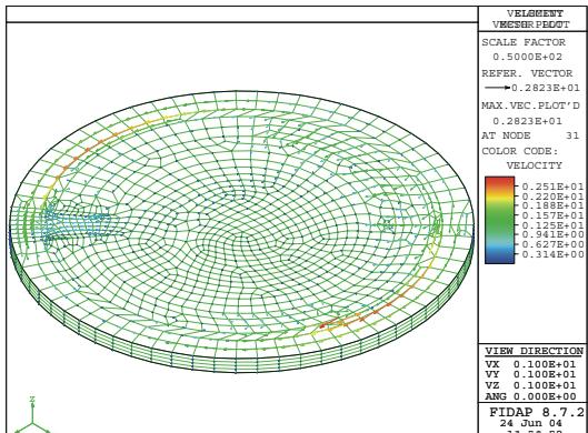
Fig. 7. Three-dimensional mesh overlayed with surface velocity vectors. Viewed from northeast.
