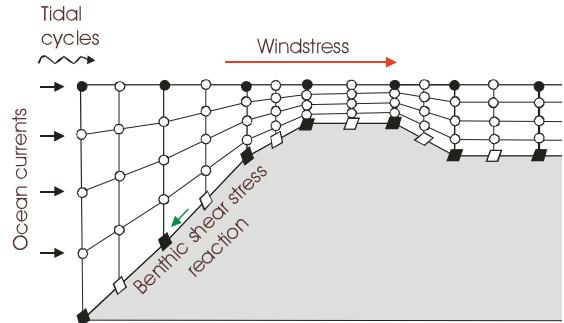
Fig. 3. Two-dimensional slice through finite elements adapted to atoll forms
