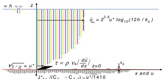
Fig. 2. One-dimensional view of flow over bottom substrates (from Peterson 1999)
