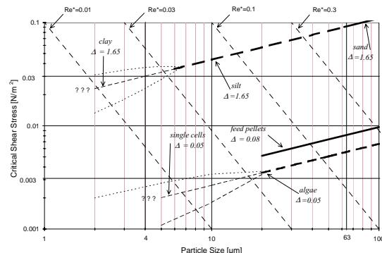
Fig. 1. Measure of substrate quality under tropical seawater. The relationship between hydrodynamics (expressed as benthic shear stress) and re-suspension of feed and plankton (as organic matter of various sizes), and also soil and sediment (classified as mineral particle sizes “sand”, “silt”, and “clay”). Various morphologies of coral colonies could be plotted on this sort of chart, albeit larger sizes & stresses.
