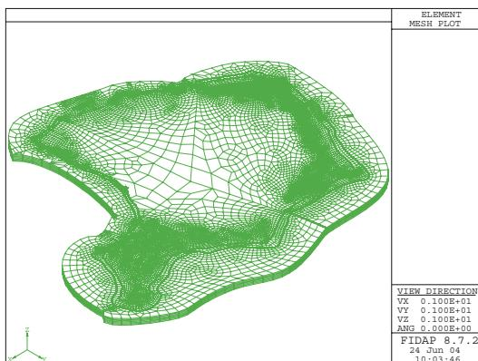
Fig. 10. Finite element mesh developed for Rongelap (isometric view from northeast)
